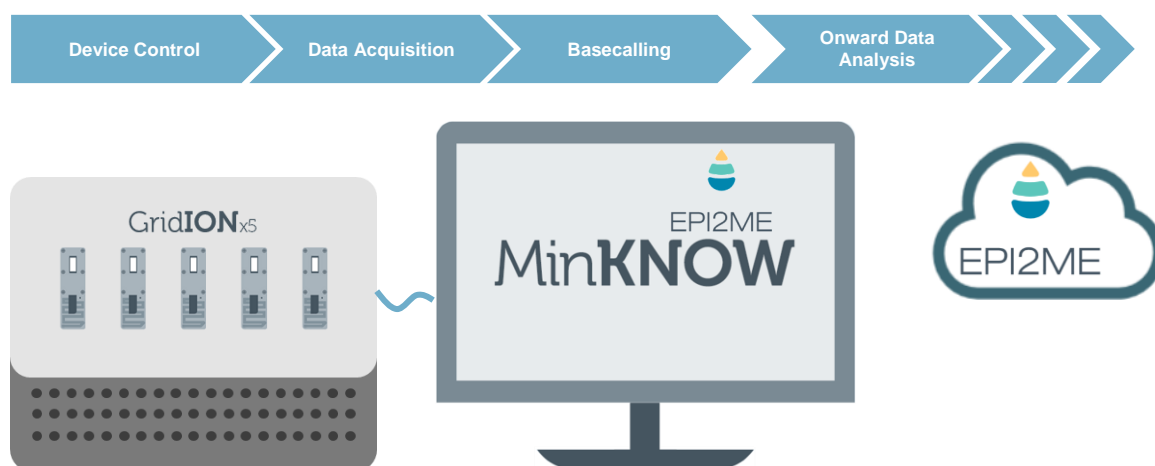
Figure 1: Default data analysis workflow of the GridION device
