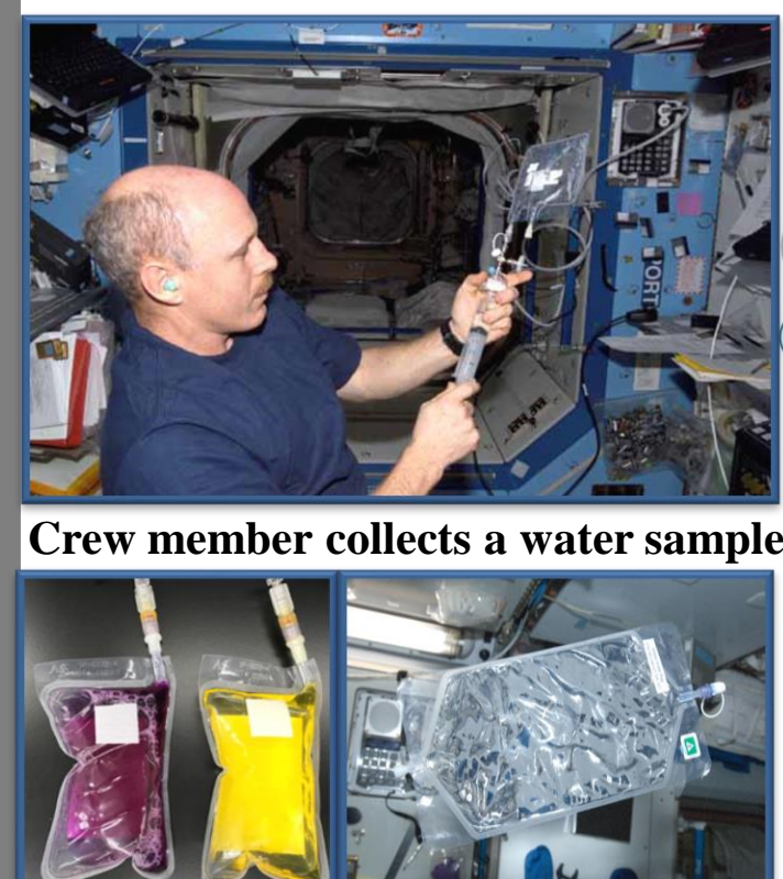
Coliform indicator bag (in-flight) and post-flight analysis bag (returned to ground for analysis)
