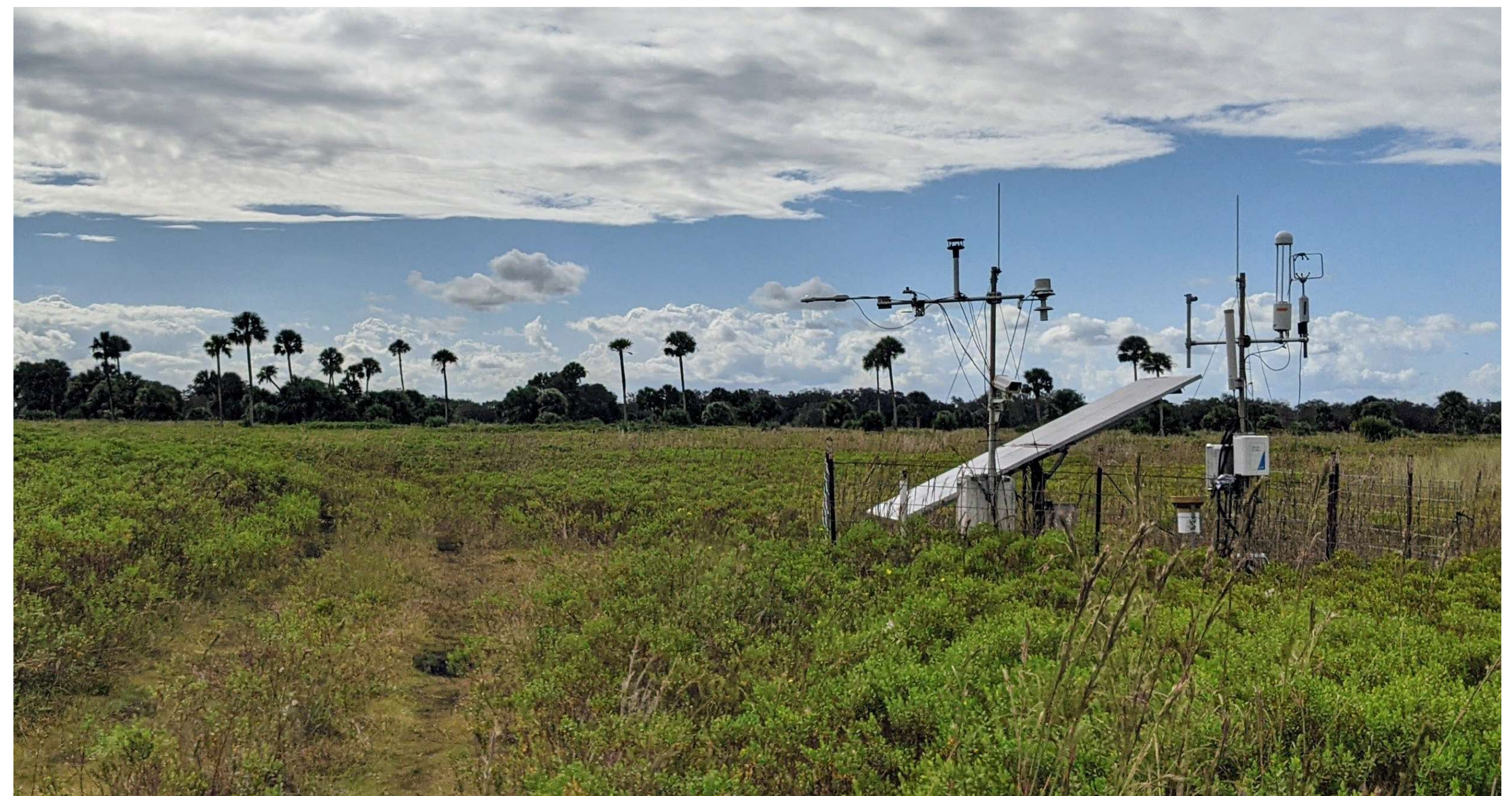
Fig.2 Eddy covariance flux towers capture micro-meteorological data such as: air temperature, humidity, wind velocity, net incoming radiation and more
