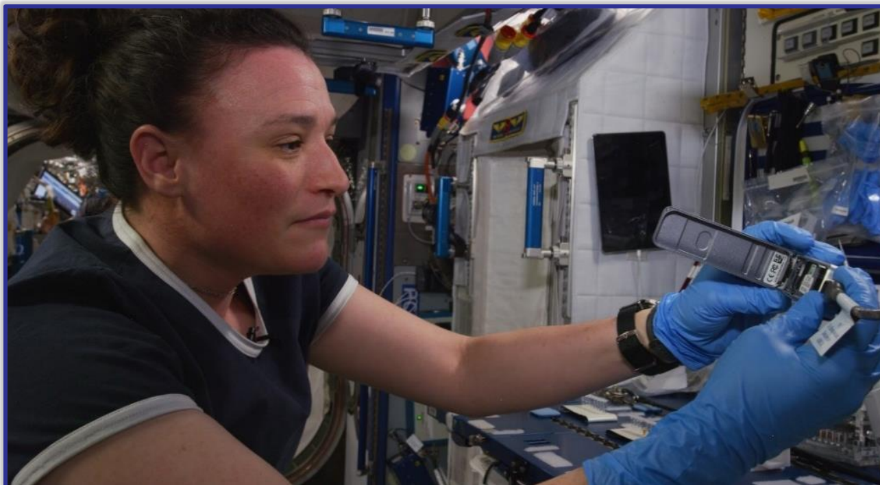
Figure 2: Astronaut Dr. Serena Auñón-Chancellor holding the MinION Mk1B onboard the ISS. The MinION is being used by NASA for both culture-dependent and culture-independent microbial identifications.
